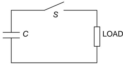
Figure 1.1: basic pulse generator topology
