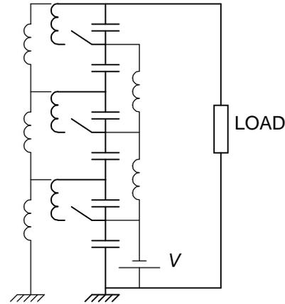
Figure 2.7:3 stages 'Fitch' pulse generator
