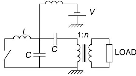
Figure 2.6: resonant charge circuit with and without step-up transformer
