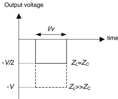
Figure 3.6: Self-Matched line pulse waveform
