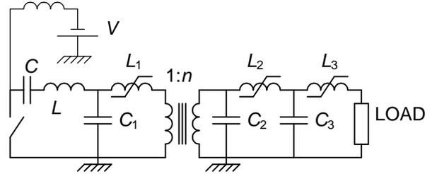
Figure 2.4: Magnetic Pulse Compression Topology
