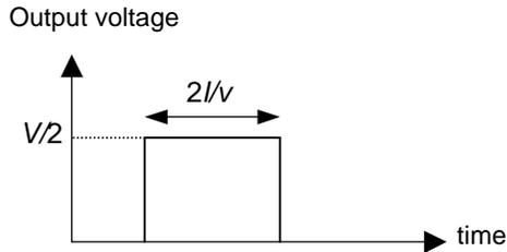
Figure 3.2: transmission line pulse waveform
