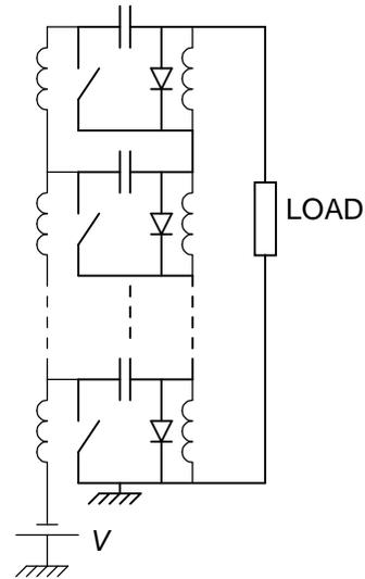
Figure 1.6: 'Solid-State Marx' Adder Topology
