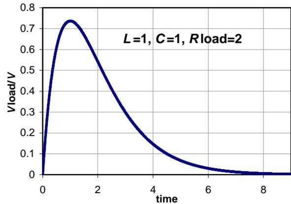
Figure 2.2: pulse waveform on a resistive load in critically damped condition
