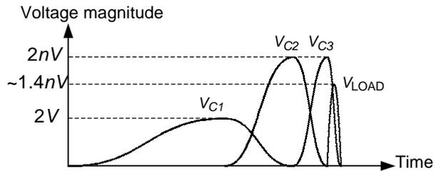
Figure 2.5: pulse propagation in the compression stages
