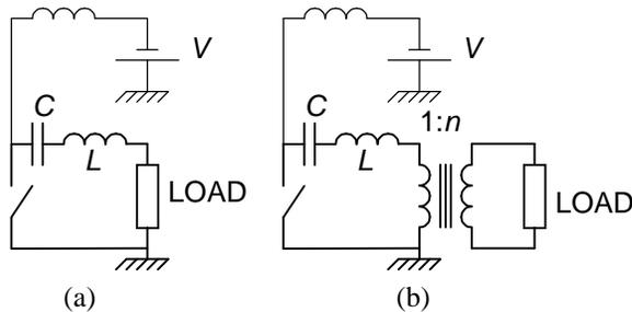
Figure 2.1: basic resonant charge circuit with and without step-up transformer
