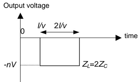
Figure 3.10: Blumlein-Fitch pulse waveform
