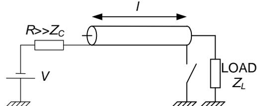
Figure 3.3: alternative transmission line discharge ( $Z_L = Z_C$ )
