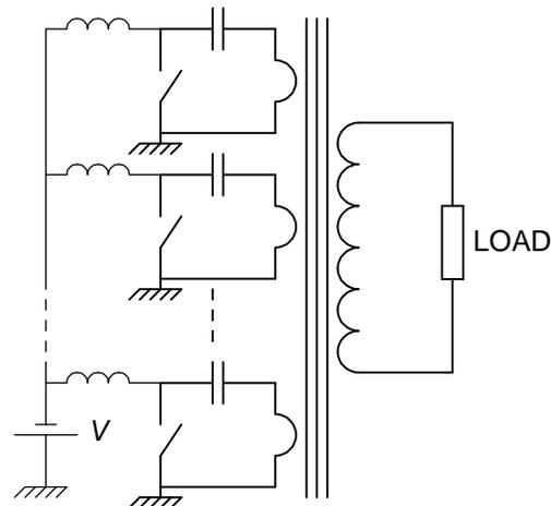
Figure 1.3: Pulse transformer Topology
