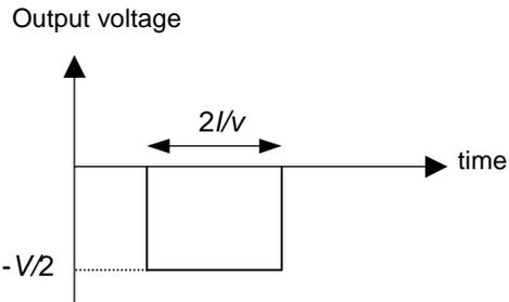
Figure 3.4: transmission line pulse waveform
