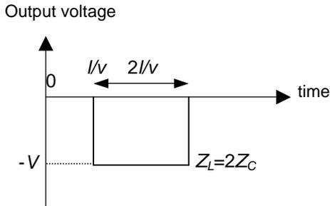
Figure 3.8: Blumlein pulse waveform
