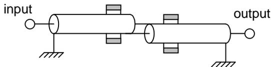
Figure 4.2: Pulse polarity inverter
