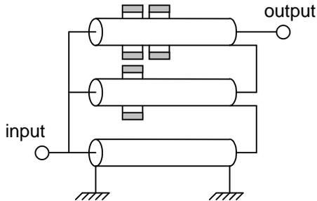
Figure 4.1: 1:1:3 transmission line pulse transformer
