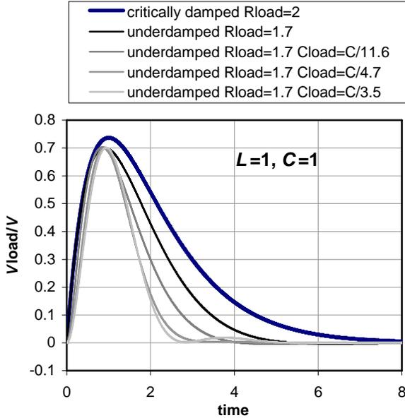
Figure 2.3: pulse waveform optimization to shorten the pulse length
