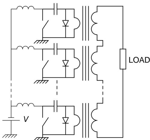
Figure 1.4: Series Pulse Transformers Topology
