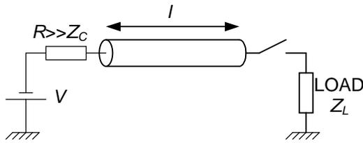
Figure 3.1: basic transmission line discharge
