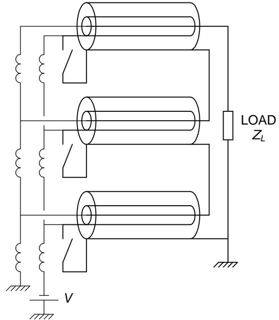
Figure 3.9: Three stages Blumlein 'Fitch' pulse generator
