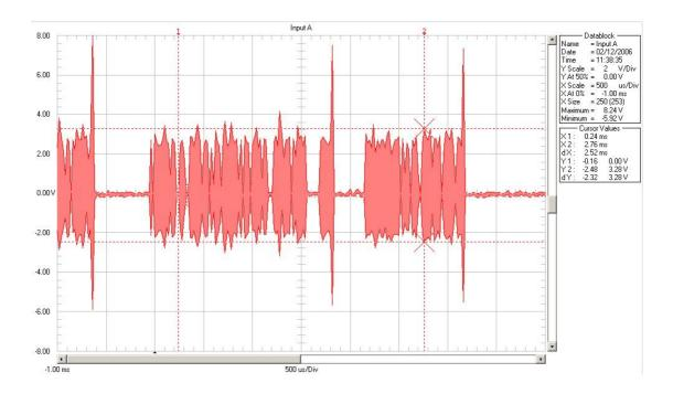
If we "zoom" in, we can see better what is happening. Each pulse creates a resonant signal/ringing in the collector. When the signals from each 3 frequencies mix at the right point, a ring which is much larger results.
