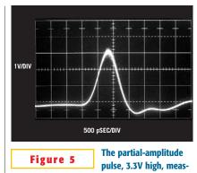
ures 700 psec wide with a 1.25-nsec base. The trace granularity is an artifact of the 3.9-GHzsampling-oscilloscope operation.
