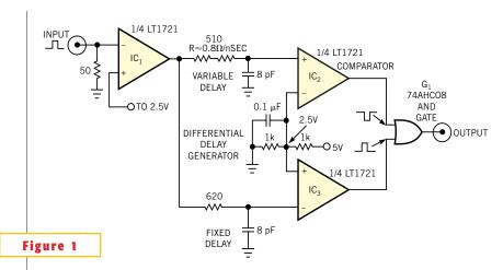
This pulse generator has 0- to 10-nsec width and 520-psec transitions.  $IC_1$  unloads termination and drives the differential delay network. The  $IC_2$ - $IC_3$  complementary outputs represent delay difference as edge timing skew.  $G_1$ , which is high during  $IC_2$ - $IC_3$ 's positive overlap, presents circuit output.
