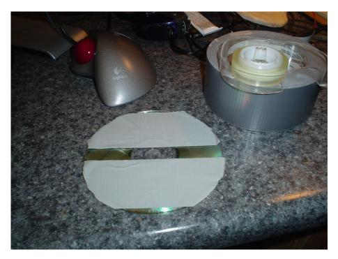
For the wire, any type will work as long as it will stick to the duck tape. Place the CD into the empty CD holder. Take about six inches of the end of wire, make a right angle bend in it, and tape it to the hub of the CD holder to secure it while winding. Your setup should look something like the following:
