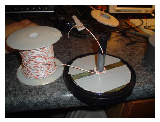
After securing the wire to the center hub, slowly turn the CD with the holder and press the wire gently onto the tape to form the spiral. Try not to put any tension on the wire as the tape will hold it in place. Once finished, the winding should look something like this:
