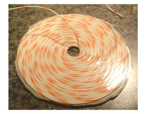
First, take the CD and cover one side of it with strips of double-sided sticky tape. Try to cover as much of the surface as possible without overlapping the strips. Now place strips of duck tape on top of the double-sided sticky tape so that the sticky side of the duck tape is facing upwards. This will be used to adhere the wires to the CD while winding the coil.
