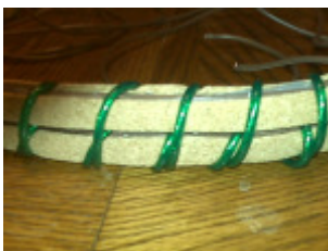
First winding of control coils around first collector. All wound Counter Clockwise.
