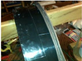
Lamp Chord is separated. First winding of three turns takes place, glued to the cork. This is the INNER loop of the collector. The second winding is then glued on top of this. This is the OUTER loop of the
