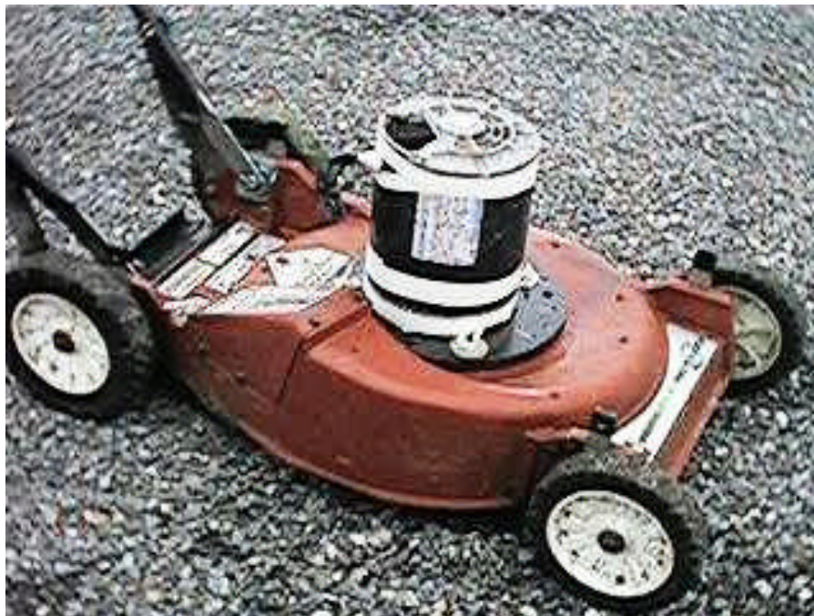
Dougs converted lawn mower to run in RV modes with motor attached on top.
