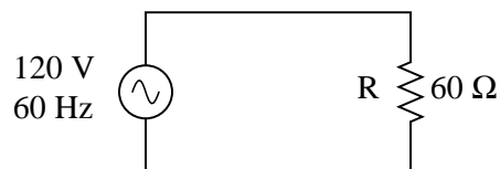
Figure 11.1: Ac source drives a purely resistive load.
