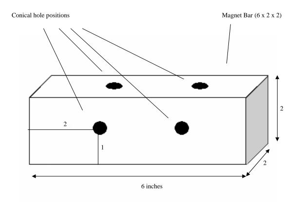
Apposing conical holes are also similarly positioned on the magnets opposite sides.
